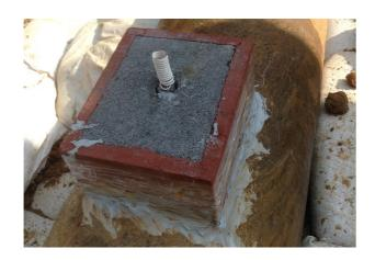
TSID Blocks are designed to fit common ammunition profiles to ensure intimate contact but they can be further contoured by the user where required. They are initiated electrically using a Disarmco Thermite Initiated Starter (TIS); which is inserted into the block.
